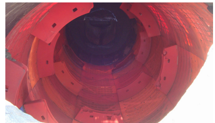
Smaller pieces of material filter through screen openings and larger continues to the discharge end.
