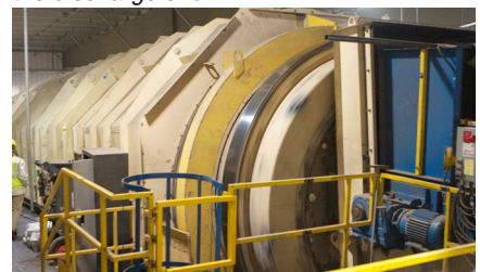
Rotary Trommel Screen cylinders are perfectly concentric, eliminating vibration and wobbling.
