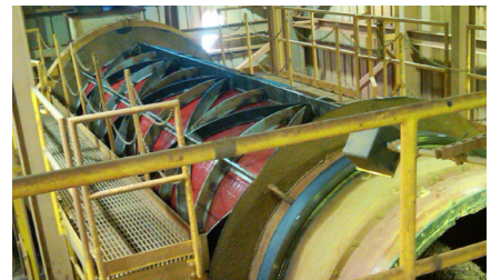
Rotary Trommel Screens are used in mineral processing, MSW and other industrial processes.
